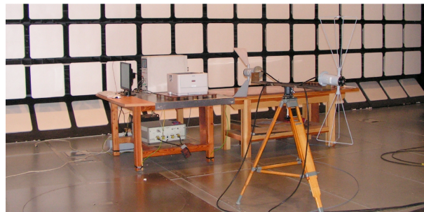
Figure 7. Measuring system inside of the anechoic chamber.
