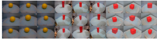
Figure 3. Nine sample views out of 72 views of the objects with known shapes, sphere, prism, and cube [25], acquired using a multiple-camera setup.
