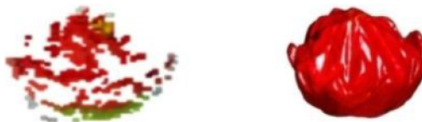
Figure 12. Left: Point cloud obtained for the lotus object using VisualSFM [26], right: a 3D model of the lotus obtained using the proposed method.
