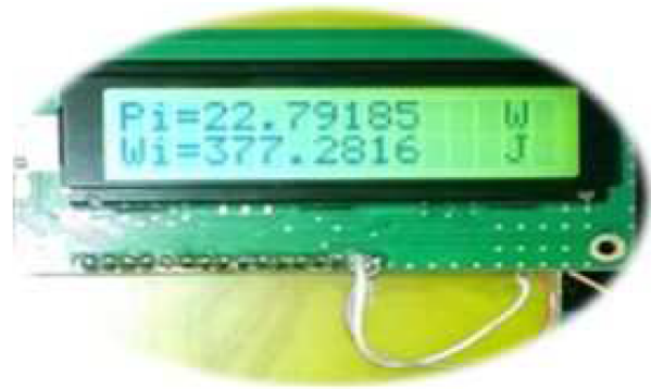
Figure 8. The active power and the energy values measured by PIC 16F877.
