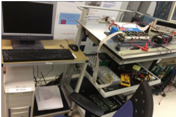
Figure 22. Experimental RT LAB platform with the power converter system.
