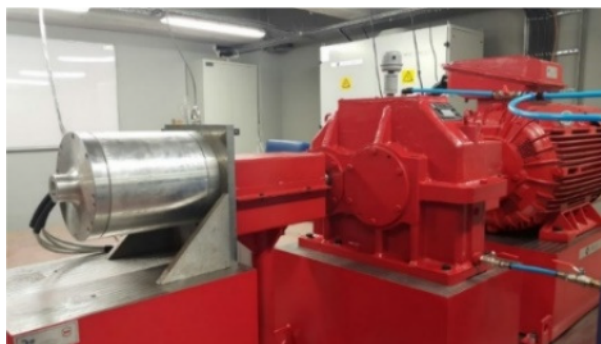
Figure 9. Experimental test bed (150 kW, 400 Nm).
