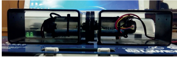
Figure 2. Expanded view of the motor/generator coupling.
