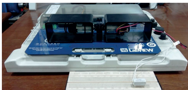
Figure 1. DC motor control trainer.
