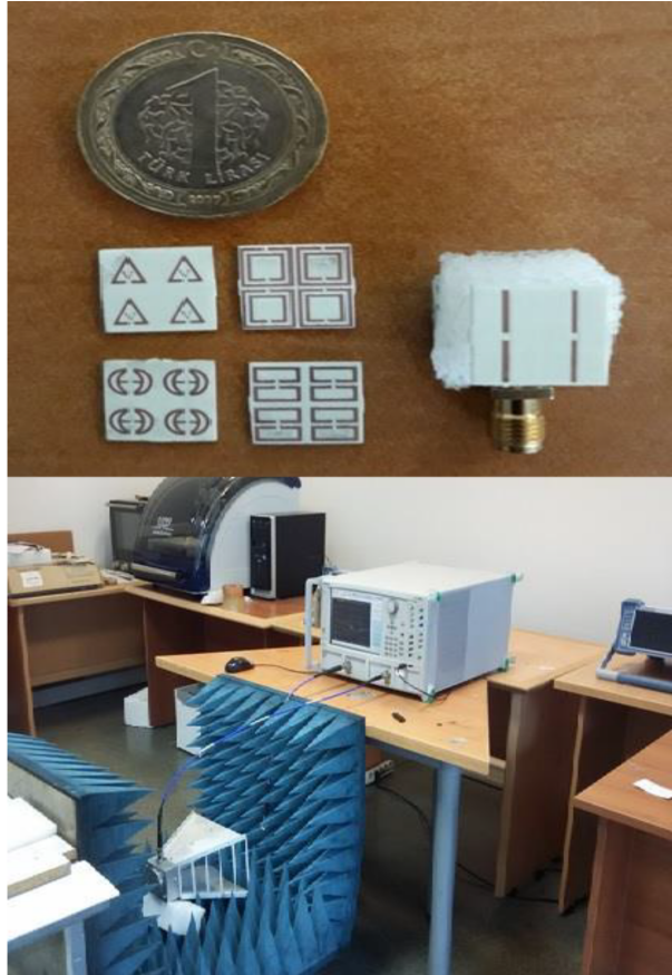
Figure 8. Photograph of fabricated prototype of MMs and measurement setup.
