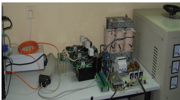
Figure 4. Experimental setup of the D-STATCOM.
