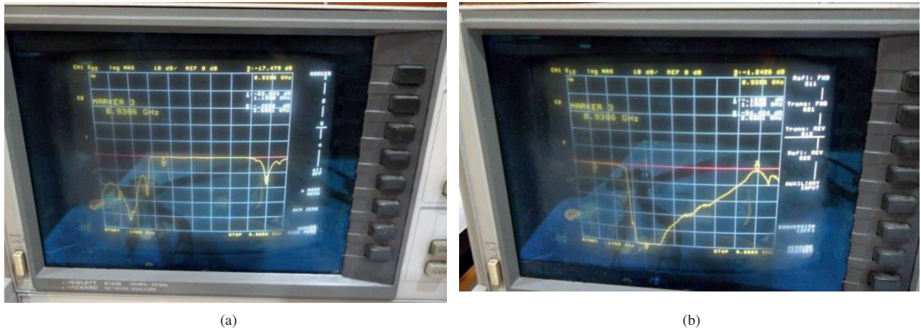
Figure 16. The measured S -parameters of the proposed LPF with an HP8720B network analyzer. (a) S_{11} and (b) S_{21} .
