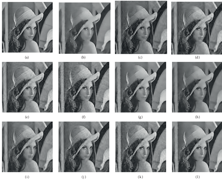
Figure 7. Denoised Lena image using various methods for \sigma = 30 : a) clean, b) NLM, c) BayesShrink, d) NeighShrink, e) NeighSUREShrink, f) EBF, g) ANLM, h) NLM+BayesShrink, i) NLM+NeighShrink, j) NLM+NeighSUREShrink, k) EBF+NeighSUREShrink, and l) ANLM+NeighSUREShrink.
