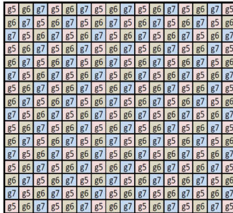
Figure 2. Bit-plane selection approach for a 16 \times 16 block presented in [16].
