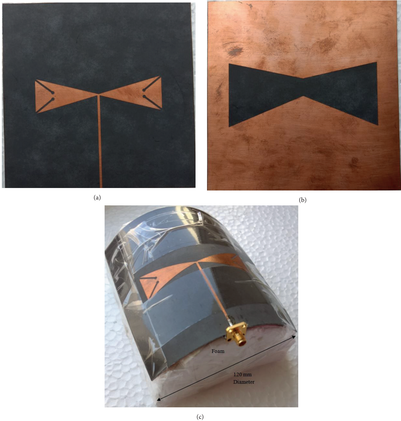
Figure 9. Photograph of prototype fabricated antennas: (a) front view of the proposed planar antenna, (b) back view of the proposed planar antenna, and (c) top view of a proposed cylindrical conformal antenna with 60-mm radius of curvature.
