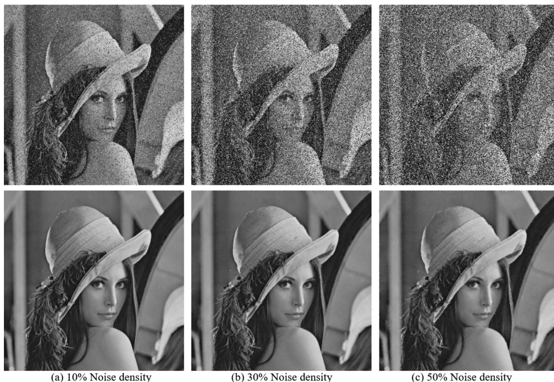
Figure 6. Filtering results using the proposed image with three different noise densities.
