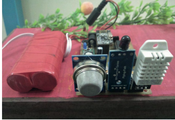
Figure 10. Final fire detection WSN node in working environment.
