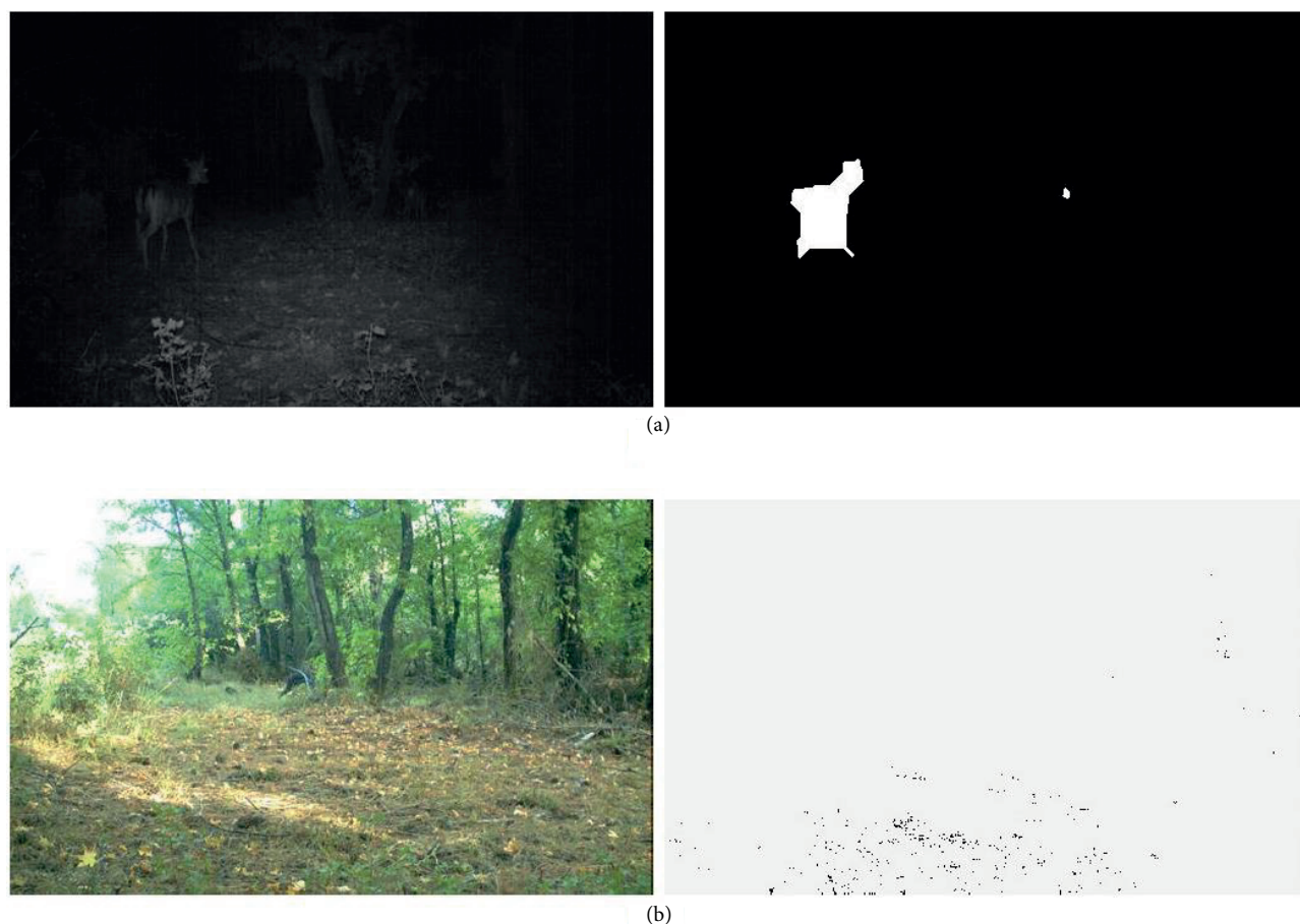
Figure 7. A successful (a) and a failed (b) example of detecting animals with background subtraction. Images on the left are two consecutive images in raw camera-trap dataset. Since the difference between images is too much, the background subtraction result of the second image implies that the image has an animal while it does not.
