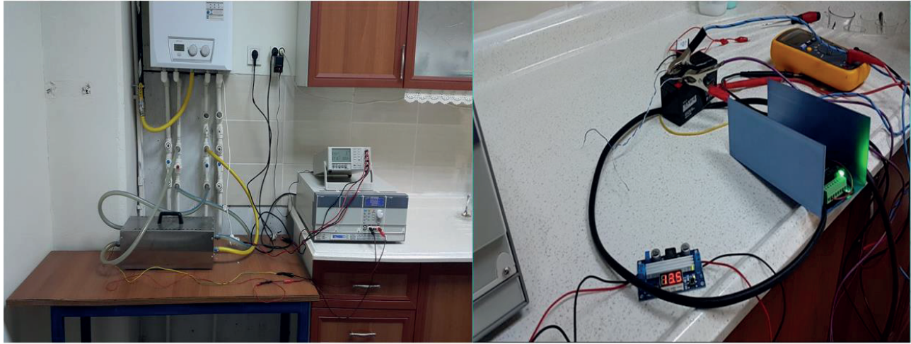
Figure 4. Connection of the combi generator and the experimental setup.
