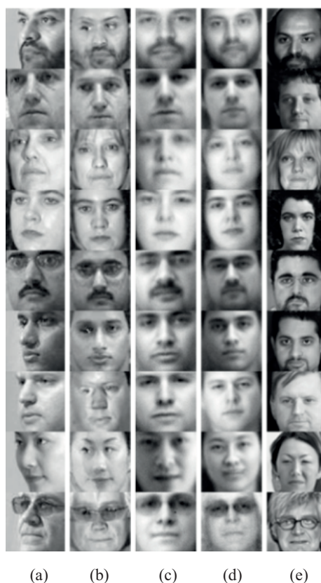
Figure 9. (a) 2-D-aligned posed image, (b) 3-D model-based method [11], (c) SDAE-based method, (d) [11] enhanced by SDAE, (e) GAN-based method [15].
