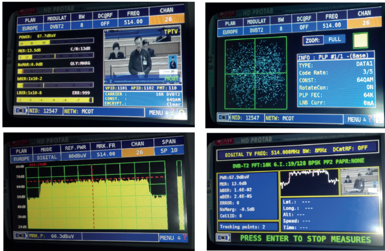
Figure 5. Display from the DVB-T2 signal analyzer.
