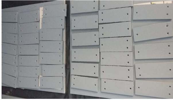
Figure 1. Rectangular porcelain samples coated by RTV silicone rubber.
