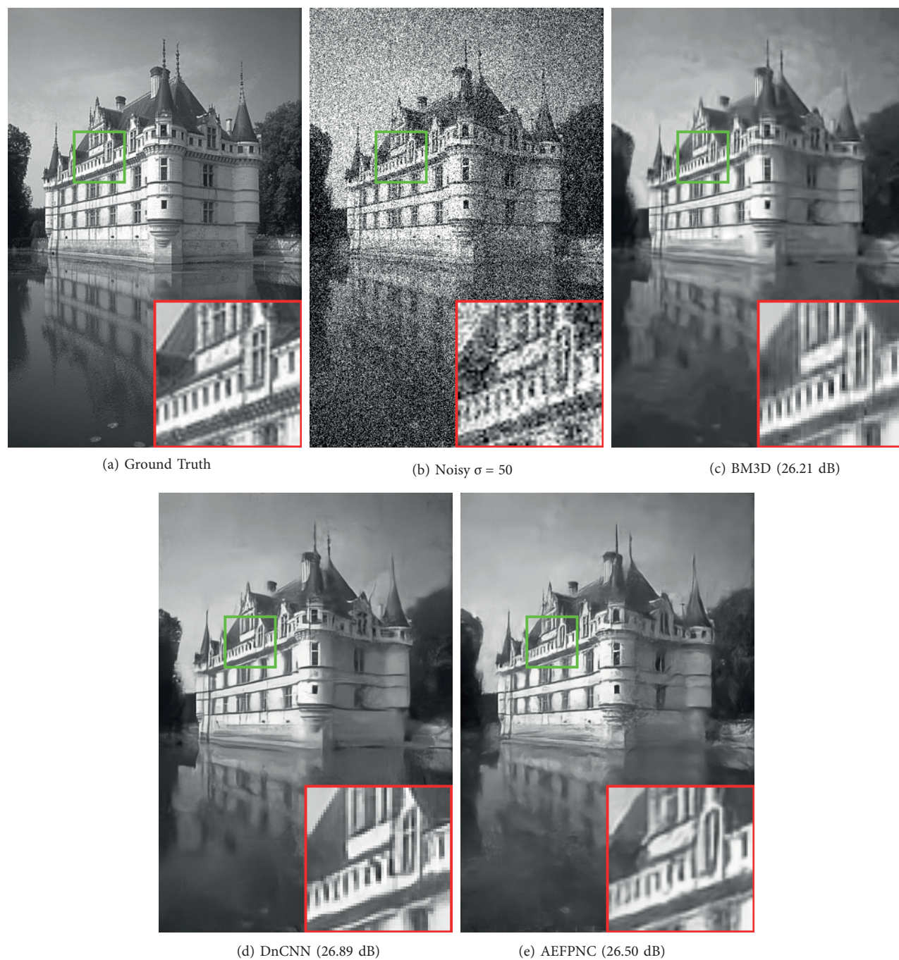
Figure 5. Grayscale image denoising results of image 102061 in BSDS68 dataset with noise level \sigma = 50 . BM3D and DnCNN results are taken from [5].
