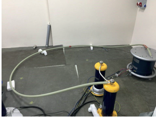
Figure 4. PD localization experiments on a XLPE HV cable.
