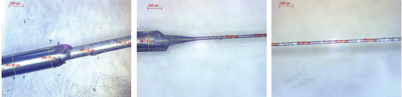
Figure 2. Image of a fabricated sensor head by chemical etching process under microscope. a) fiber with/without plastic jacket, b) etched fiber and c) another part of etched fiber.
