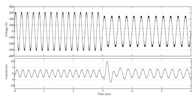
Figure 5. Output voltage and current of the 21-level hybrid MLI during the speed change of the motor.
