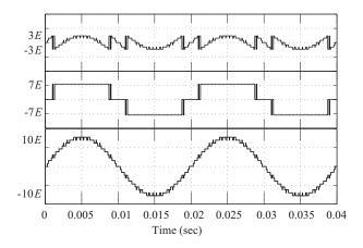
**Figure 3.** Branch voltages of: cross switch inverter  $(V_{C1} + V_{C2})$ , CHB  $(V_{C3})$  and hybrid MLI  $(V_{AB})$ .
