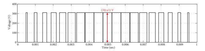
Figure 15. Common mode voltage of CHB inverter.
