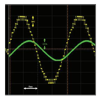
Figure 9. Experimental output voltage and current before step change at m = 1 and  $N_S = 1500$  rpm.
