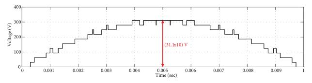
Figure 16. Common mode voltage of 21-level hybrid inverter.
