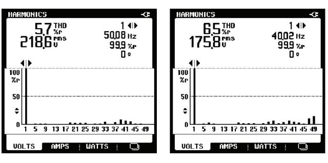
Figure 11. Experimental harmonic spectrum before step change at m = 1 and  $N_S = 1500$  rpm.
