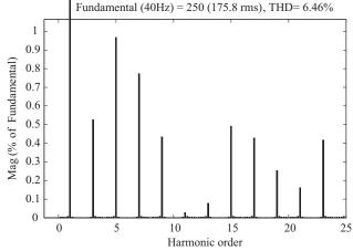
Figure 6. Harmonic spectrum before step change at m = 1 and  $N_S = 1500$  rpm.
