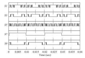
Figure 2. Gate pulses of the odd switches (S1, S3, S5, S7) and S9 of the hybrid MLI.
