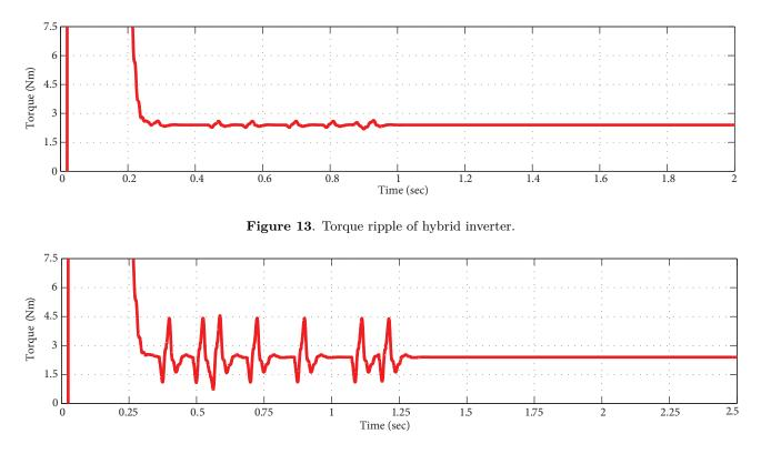
Figure 14. Torque ripple of CHB inverter.
