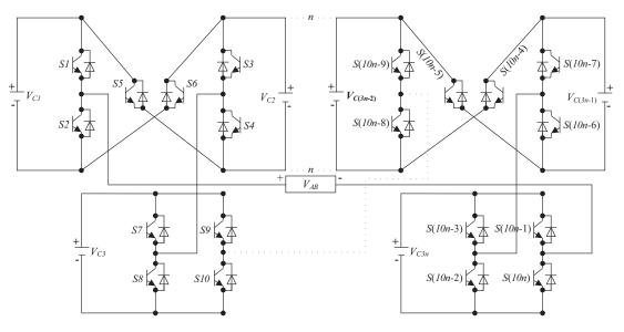
Figure 1. Schematic diagram of 21-level hybrid multilevel inverter.
