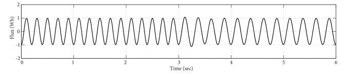
Figure 8. Constant stator flux during the step change of the motor.
