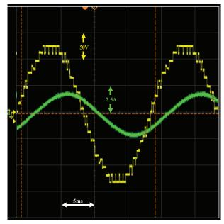
Figure 10. Experimental output voltage and current before step change at m = 0.8 and  $N_S = 1200$  rpm.
