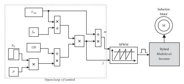
Figure 4. Control diagram of the open loop v/f motor control technique.
