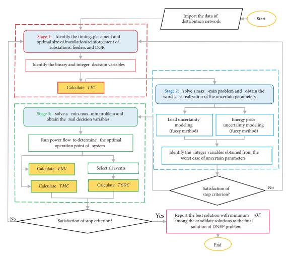
Figure 4. Flowchart of the proposed tri-stage decomposition approach for solving the DNEP problem.
