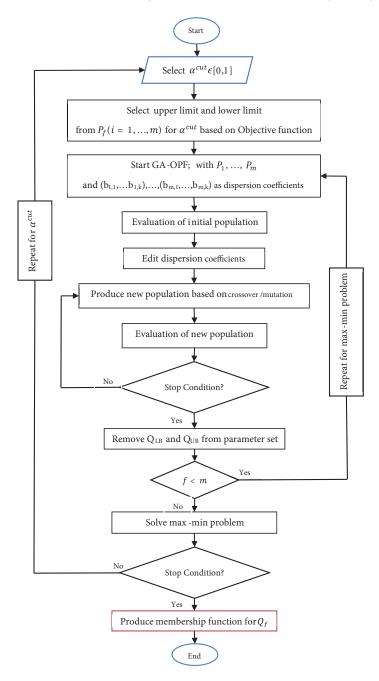
Figure 3. Process of modeling the uncertainties based on the fuzzy theory incorporation with GA-OPF algorithm.
