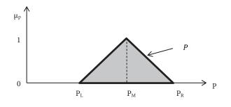
Figure 1. Graphical representation of the load as a triangular fuzzy number.
