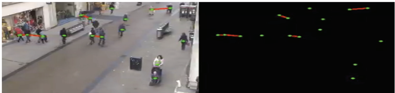
Figure 9. Distance calculation for an example frame, where pedestrians are marked using bounding box center. The distance is calculated between the center points with Euclidean distance. Our algorithm detects a violation of social distancing measures.
