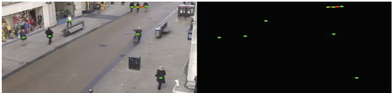
Figure 4. There is a point in each pedestrians bounding box center. In our output, we delete each person's bounding boxes on the left and put a point in the center of the bounding boxes. On the right, only those points are visible.
