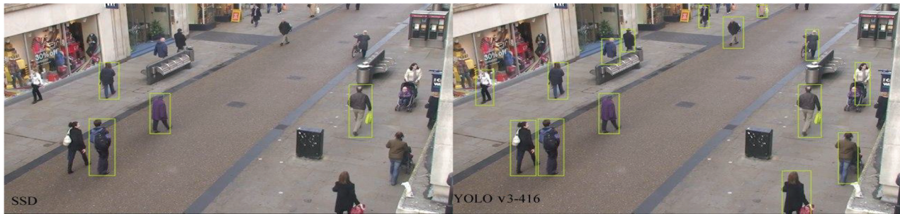
Figure 6. SSD inference (left) vs. YOLO v3 inference (right). There is a comparison of SSD and path in this visual. YOLO is seen to give better and faster results than SSD. That is the reason why no SSD was used.
