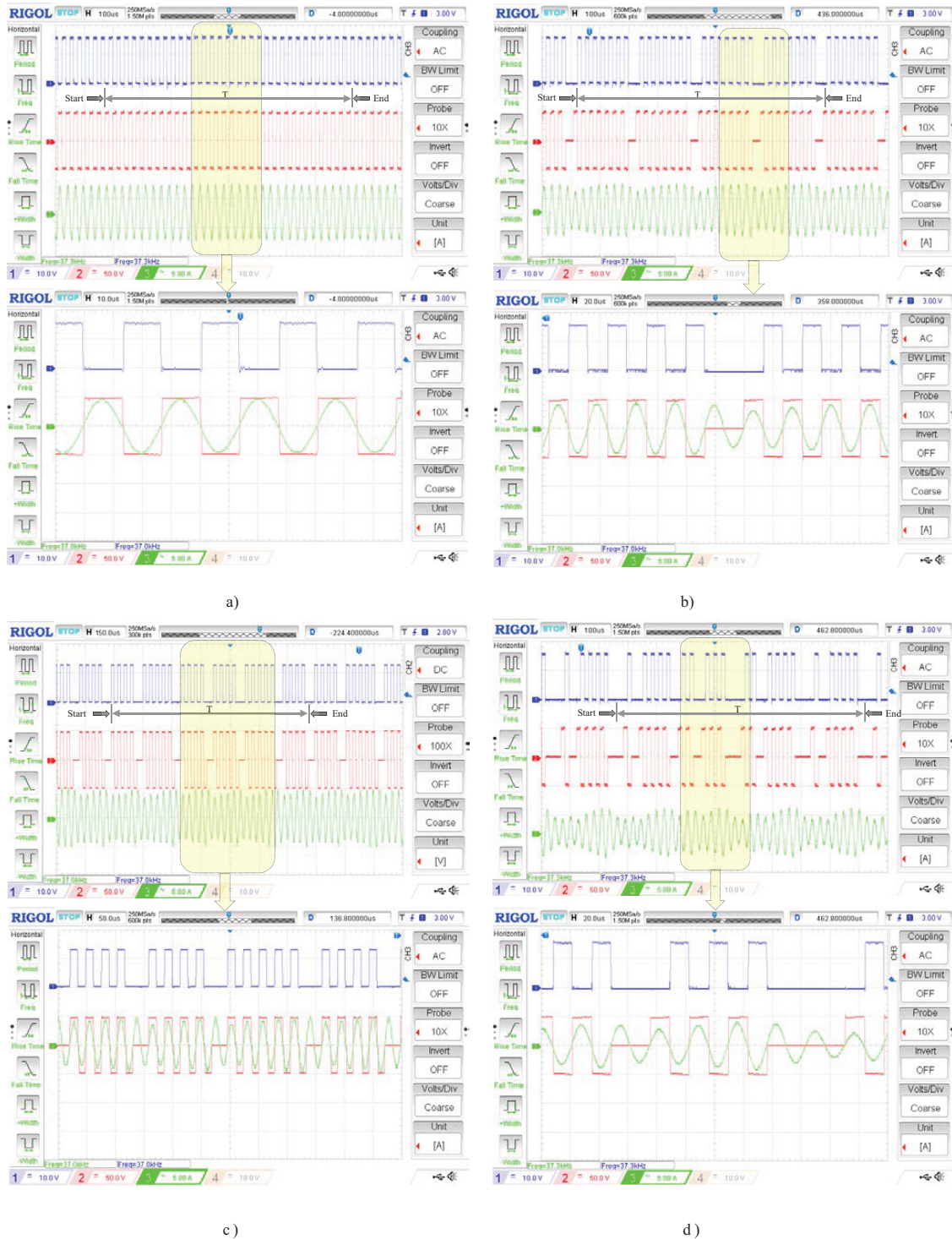
Figure 14. Experimental waveforms of Vgate (CH1), Vab(CH2), and ired (CH3) for a) N = 32, b) N = 28, c) N = 26, d) N = 21.
