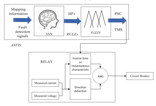
Figure 4 shows the adaptive relaying scheme using ANFIS [85]
