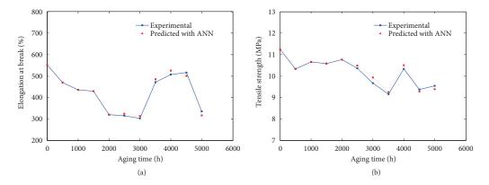
Figure 4. Experimental and predicted mechanical properties according to thermal aging time, (a) elongation at break, (b) tensile strength.
