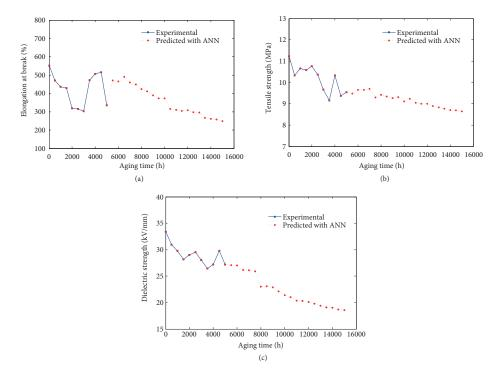
Figure 7. Experimental and predicted elongation at break, tensile strength and dielectric strength as function of thermal aging.
