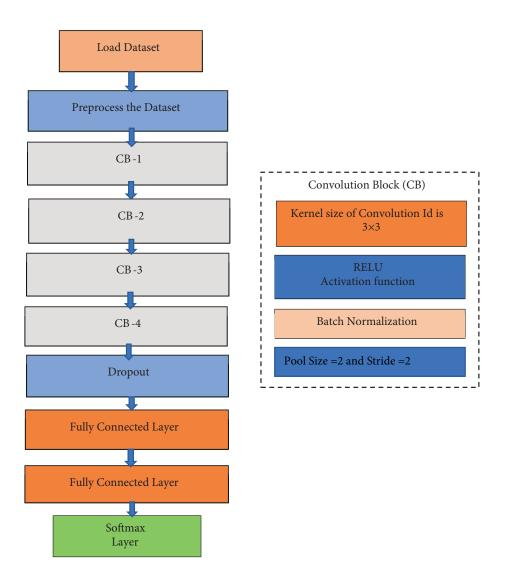
Figure 2. The overall process structure of the CNN model.
