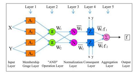
Figure 1. The illustration of the ANFIS architecture structure [40].
