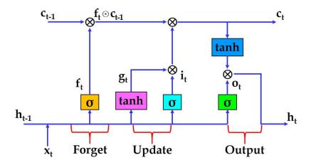
Figure 3. The structure of a single LSTM unit.
