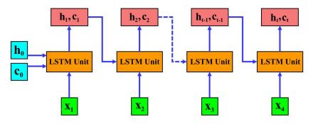
Figure 2. The architecture of LSTM network.
