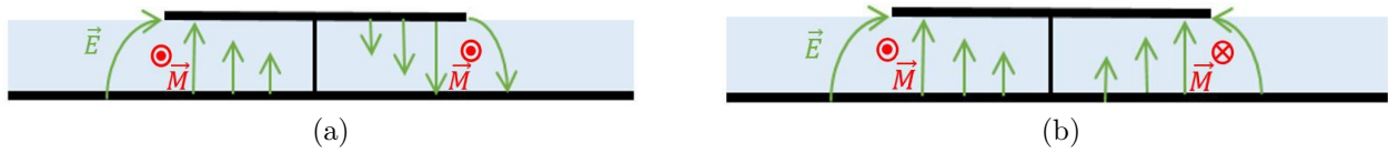
Figure 2. E-field and magnetic current distributions for (a) even and (b) odd modes.
