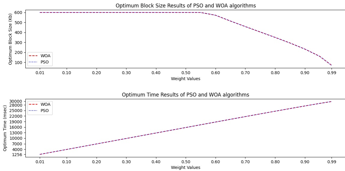
Figure 3. The relationship between the various weight values of the objective function with corresponding to the block size and total time, respectively.
