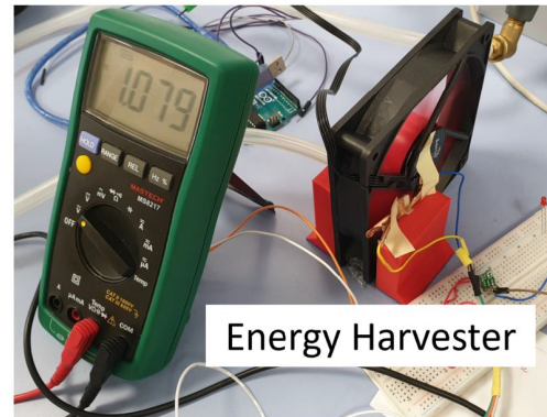
Figure 7. Frequency response plots of the circular plate: a) V_{\max} was measured as 984 mV from the wind tests, error bars are plotted from 3 consecutive trials b) The energy harvester was run under wind tests, voltage output was first validated with a multimeter.
