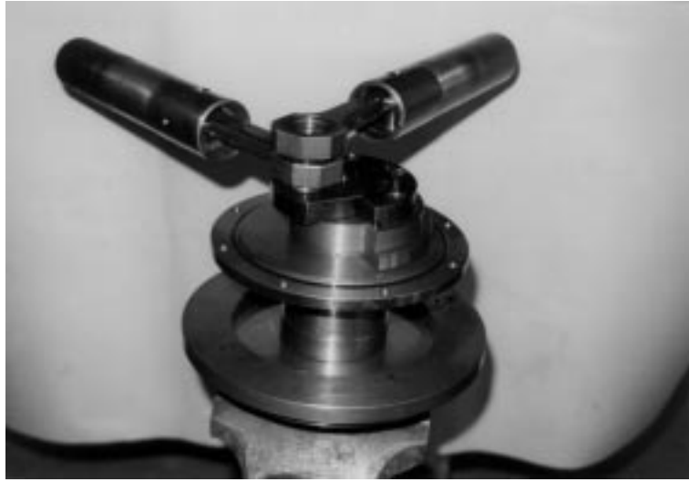
Figure 2. The crankshaft, piston rods and pistons assembly.
