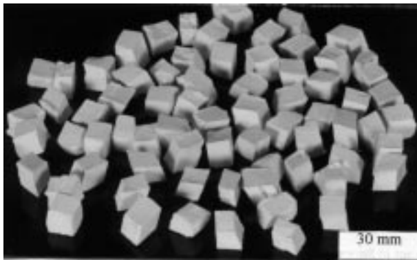
Figure 2. Feedstock pellets of the powder plus polymer mixture
