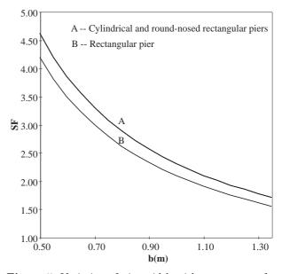
Figure 5. Variation of pier width with respect to safety factor under  $\alpha$ =0.999 level
