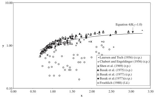
Figure 2. Relationship between y and x for non-cylindrical piers
