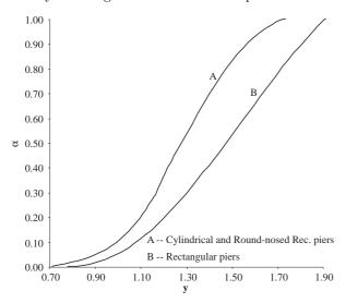
Figure 3. Variation of reliability with respect to resistance under  $\theta = 0^{\circ}$
