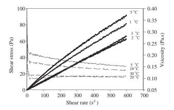
**Figure 3.** Viscosity (lines) and shear stress (symbols) of 19.5°Brix WPI-G solution at different temperatures.
