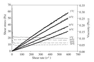
Figure 2. Viscosity (lines) and shear stress (symbols) of 18.0°Brix WPI-G solution at different temperatures.
