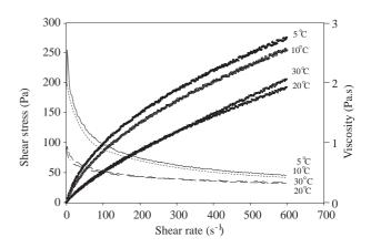
Figure 4. Viscosity (lines) and shear stress (symbols) of 21.5°Brix WPI-G solution at different temperatures.
