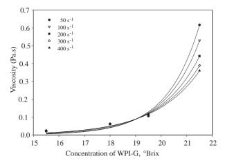
Figure 5. Effect of concentration (°Brix) on apparent viscosity of WPI-G solutions at 20°C and different shear rates.
