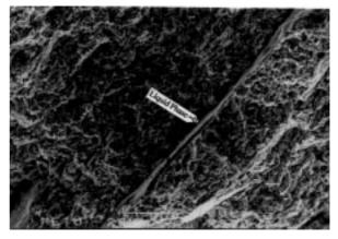
Figure 10. SEM micrograph of sample compacted at 600 MPa and sintered at  $700^{\circ}$ C for 5 h.
