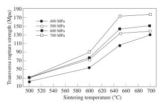
Figure 6. Relationship between sintering temperature and transverse rupture strength.
