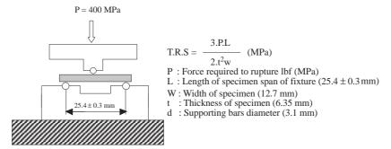
Figure 2. Transverse rupture test apparatus.
