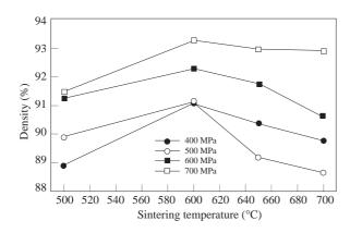
Figure 5. Relationship between sintering temperature and density of samples.
