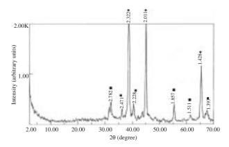
Figure 8. XRD result of the samples compacted at 600 MPa and sintered at 650°C. ♦ Al, ■ Al<sub>4</sub>C<sub>3</sub>,
