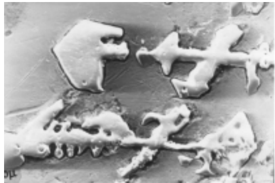
Figure 4. Faceted growth in furnace-cooling (Scale bar = 40 \mu\text{m} ).
