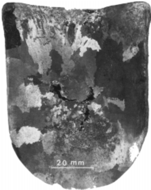
Figure 1. Large grains in a furnace-cooled ingot (Scale bar = 20 mm).
