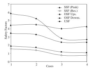
Figure 3. Safety factors for all load combinations of data set 1.
