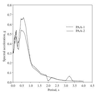
Figure 1. Whittier Earthquake - spectral acceleration.
