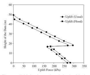
Figure 4. Uplift distribution along the height of the dam.
