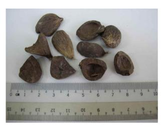
Figure 3. Various shapes of OPS aggregate.
