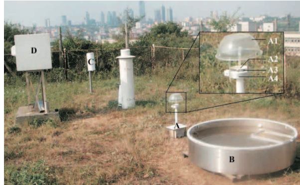
Figure 1. Location of measurement elements in the observation station. A: Naphthalene holder (A1: Transparent shelter, A2: Naphthalene, A3: Carton cup, A4: Holder for shelter and naphthalene block), B: Class-A pan, C: Rain gauge, D: Precision balance (inside the box).
