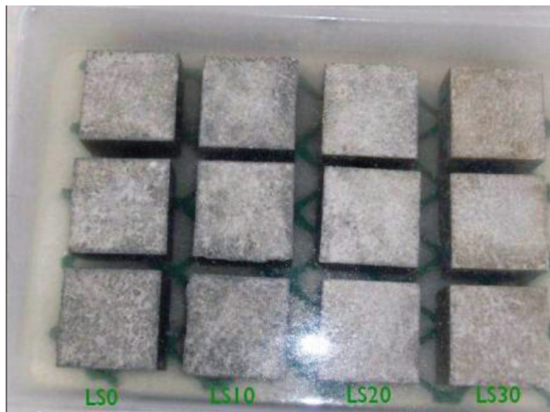
Figure 4. Mortar cubes (50 mL) cured in tap water for 360 days at 5 °C.
