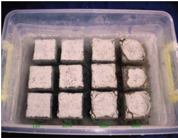
Figure 2. Mortar cubes (50 mL) exposed to 5% magnesium sulfate solution for 360 days at 5 °C.
