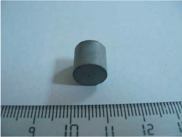
Figure 11. Macrograph of sintered TiNi compact without residual MgO.
