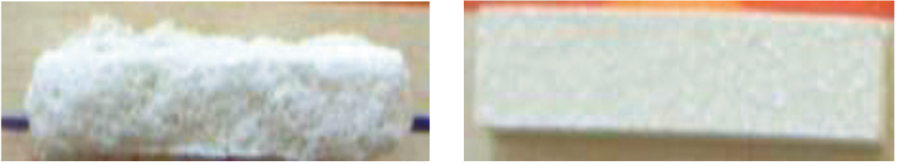
Figure 4. a) Bloating in MS-3 at 1200 °C, b) no bloating in MS-3 at 1100 °C.
