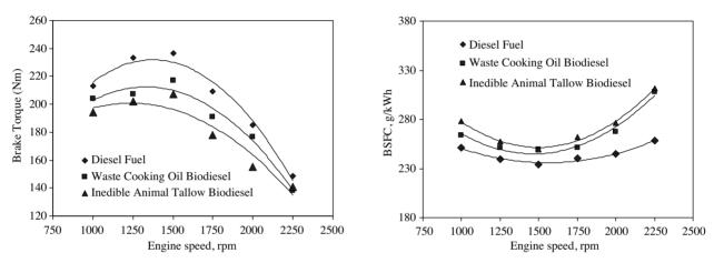
Figure 2. The variation in brake torque using biodiesels and diesel.
