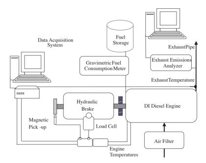
Figure 1. Schematic diagram of the experimental setup.
