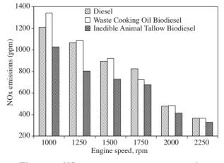
**Figure 5.**  $NO_x$  emissions versus engine speeds.
