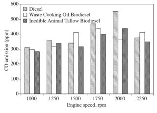
Figure 4. CO emissions versus engine speeds.
