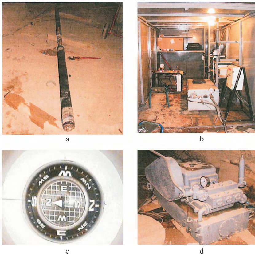
Figure 5. Some of the hydraulic fracturing test equipment. (a): Double packers; (b): Control room; (c) Borehole compass; (d): Main pump.
