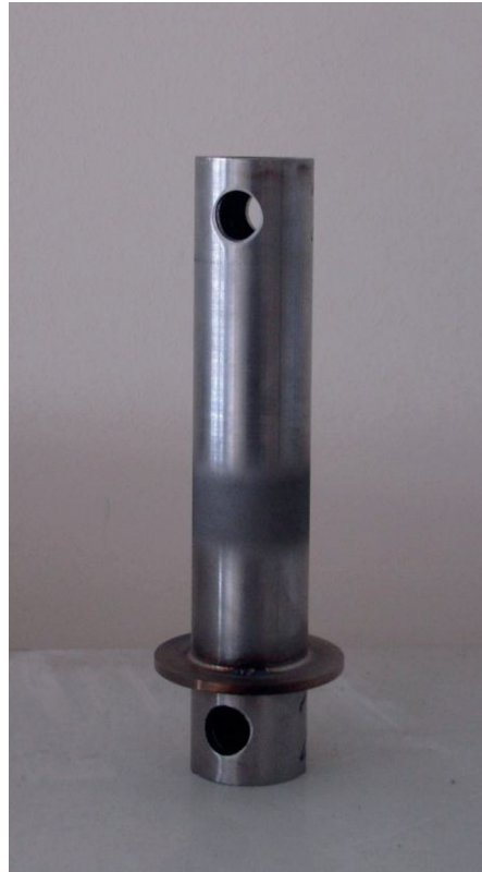
Figure 4. A sample after testing for 20 h at room temperature. Note that particles blown onto the sample cover a distance of approximately 25 mm. A collar close to the lower end of the sample is firmly fitted to the sample, diverting the abrasive particles away from the pin coupling.
