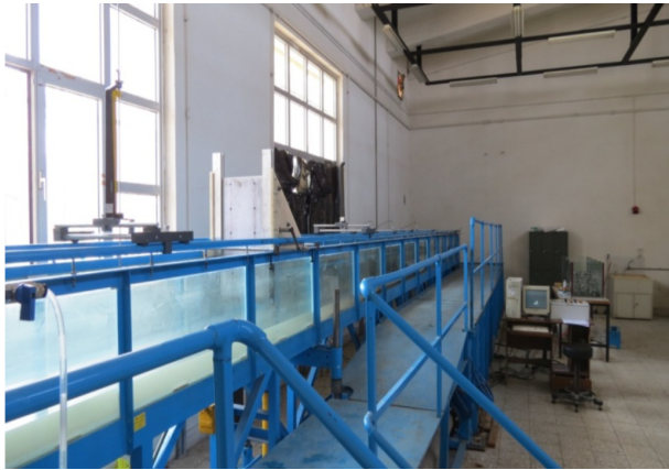
Figure 1. A view of the flume, measurement tools, and wave-producing system.
