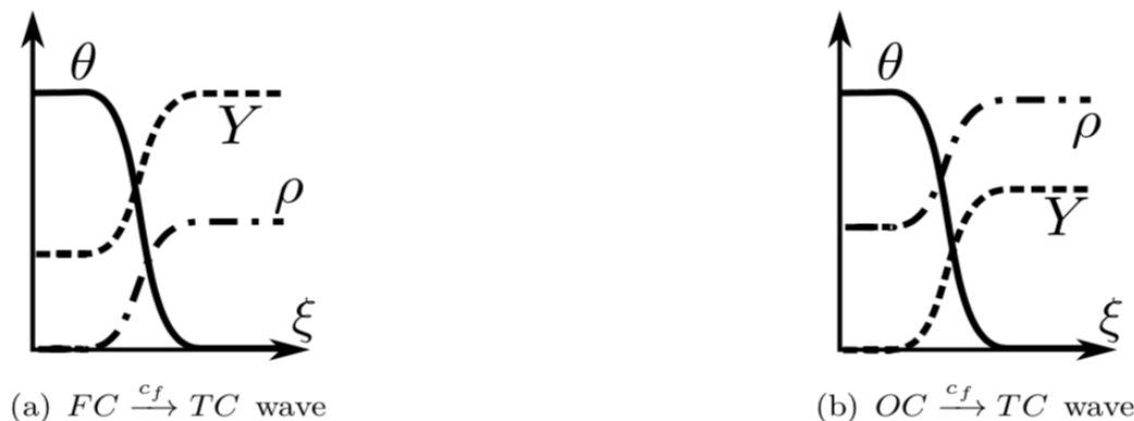
Figure 1. Fast combustion waves; \theta = temperature, \rho = solid fuel concentration, Y = oxygen concentration.
